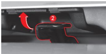
2. Lift up the hood latch lever(②) and lift up the hood
